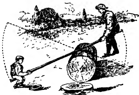
FIG. 98. A little boy on the long end of the see-saw balances a heavier boy on the other end.
